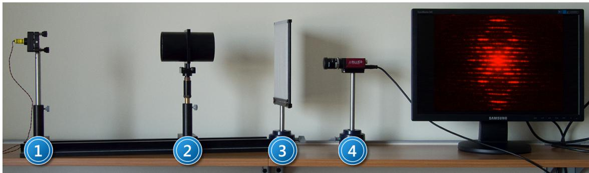
Picture 1. Measuring system for the optical simulation of  $\beta$  – DNA X-ray diffraction:
